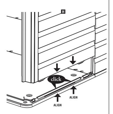
Install Wall Connector (Q) 5 places, connecting Repeat Right Side (E) and Front Right Side (H).
